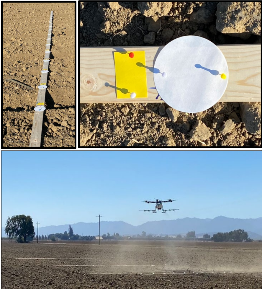
Figure 4b. Example of spray cards and filter paper placed in the field to measure swath width (Li et al 2021), also see ISO 23117-2.
